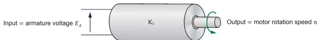
Figure 41. A dc motor can be considered to be a linear voltage-to-speed converter.
