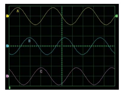
Figure 20. Oscilloscope display when channels 1, 2, and 3 of an oscilloscope are connected to phases A, B, and C, respectively, of a three-phase ac power source.
