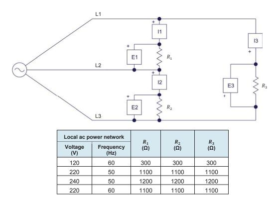
Figure 7. Delta-connected, three-phase circuit supplying power to a three-phase resistive load.
