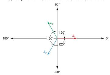
(b) Phasor diagram related to the voltage waveforms shown in (a)
