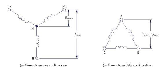
Figure 3. Types of three-phase system configurations.
