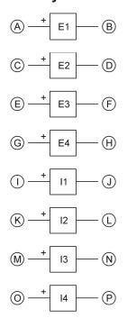
Isolated voltage and current measurement inputs
