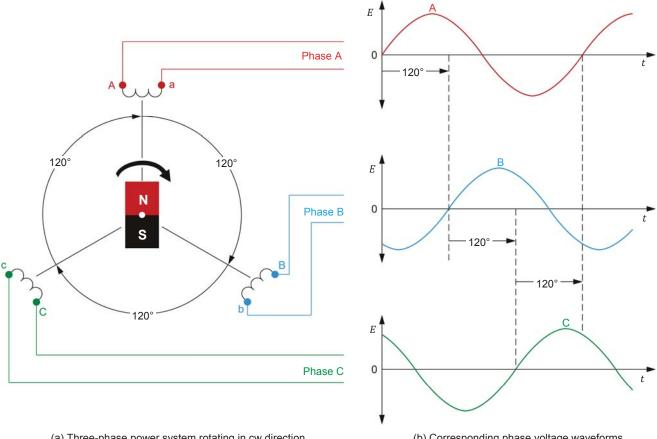
(a) Three-phase power system rotating in cw direction
