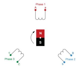
Figure 1. A simplified three-phase generator.
