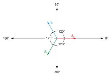
(c) Corresponding phase voltage phasor diagram
