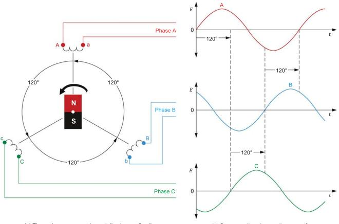
(a) Three-phase power system rotating in ccw direction
