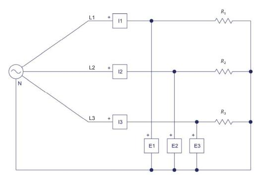
Figure 10. Three-phase power measurement using three power meters.
