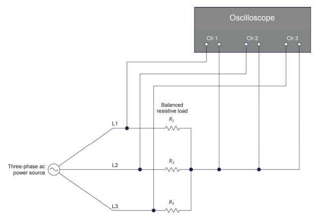
Figure 23. Oscilloscope connections to a three-wire, three-phase power system (system with no neutral wire).
