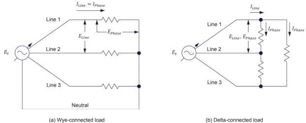
Figure 4. Types of load connections.
