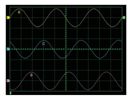
Figure 21. Oscilloscope display when channels 1, 2, and 3 of an oscilloscope are connected to phases A, C, and B, respectively, of a three-phase ac power source.
