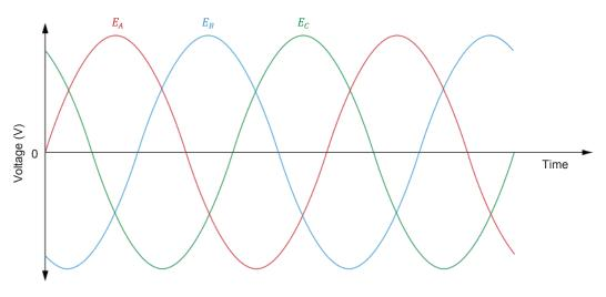
(a) Voltage waveforms produced in a three-phase ac power source
